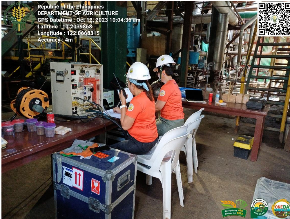
BISCOM Source Emission Sampling for PM and CO
