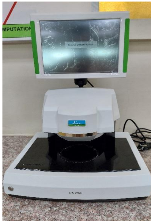
Newly-acquired NIR Analyzer for sugarcane juice analysis
